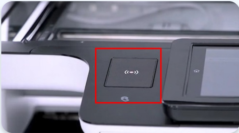
OMNIKEY RFID reader with desktop casing or industrial housing inserted into MFP enclosure
